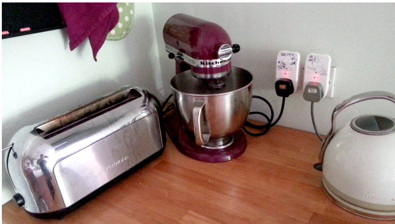
Figure 4.1: Two EDF Transmitter Plugs installed in our kitchen.
